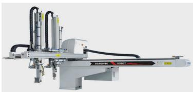
BRA700/900 Series traversing robot arm is applicable to all types of horizontal injection machine ranges of 100~300 for take-out products and sprues. Vertical arm is telescopic type, with product arm and runner arm, for two plate or three plate mold products take out. Traverse axis driven by AC servo motor. After installed this robot, the productivity will be increased 10~30%, reduce defective rate, ensure safety of operators, reduce manpower and accurately control the output to reduce waste.
